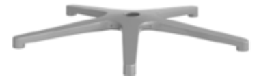
5 star die-cast aluminium base, aluminium paint finish with double coat matt transparent and anti-scratch treatment, ø 700 mm.
