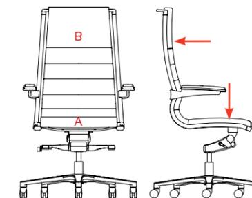
**DURABILITY TESTS ON THE SEAT AND BACK**
